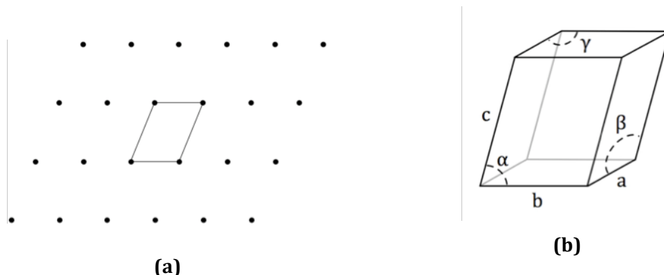
Figure 1.1: (a) Two dimensional periodic lattice with repeat unit. (b) A typical unit cell with unit cell parameters a , b , c , \alpha , \beta and \gamma .
