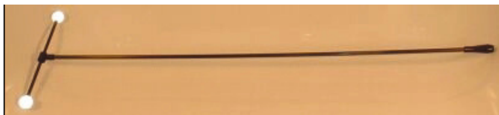
Figure 3.4. The calibration wand with 25mm retroreflective maker balls.
