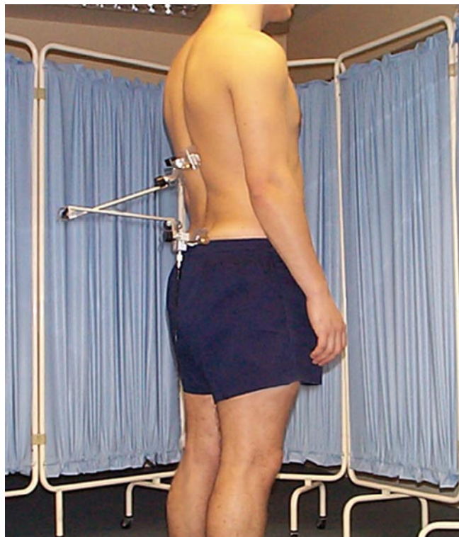
Figure 3.2. OSI CA 6000 Spine Motion Analyzer linkage (Troke et al., 2007), with permission
