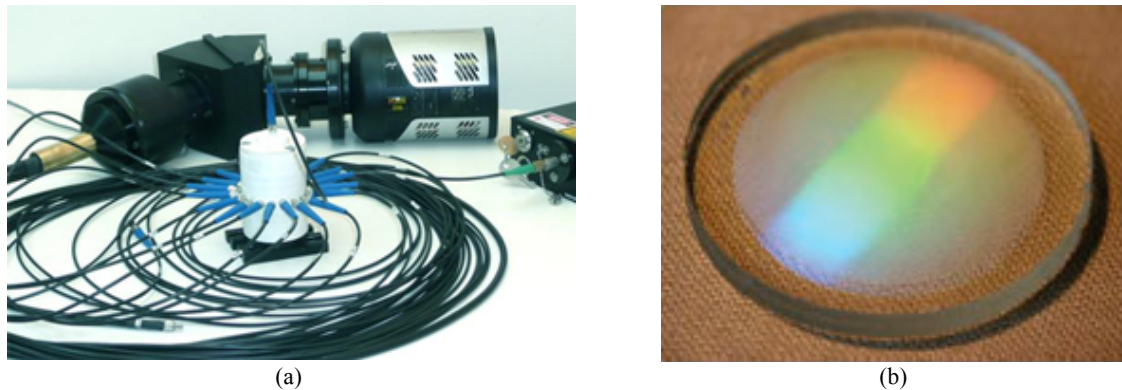
Figure 2. Multichannel spectrometer (a) and VPH transmission grating (b). Courtesy of P&P Optica Inc.
