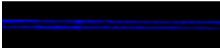
Figure 10.3: Image of a hollow core fiber filled with nematic LC 7023 taken through crossed polarizers using 464nm light. The fiber is treated with homeotropic surfactant prior to LC infiltration.
