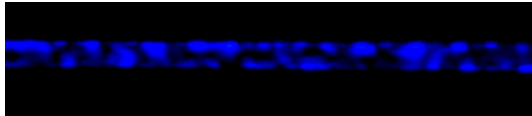
Figure 10.2: Image of a hollow core fiber filled with nematic LC 7023 taken through crossed polarizers using 464nm light.
