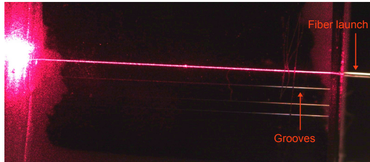
Figure 10.16: Image from above of a fiber pigtail launch into an LC filled groove heated above the N-I phase transition. The waveguide output can be seen at the far left of the picture. Total device length is \sim 12.5 mm.
