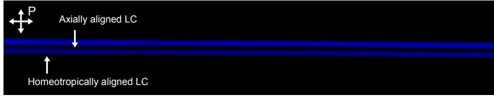
Figure 10.4: Image of a hollow core fiber filled with nematic LC 5CB. The polarizers orientations are shown in the inset denoted P.
