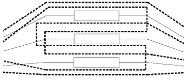
FIGURE 5.16: Water pipe layout in cooled joint bay
