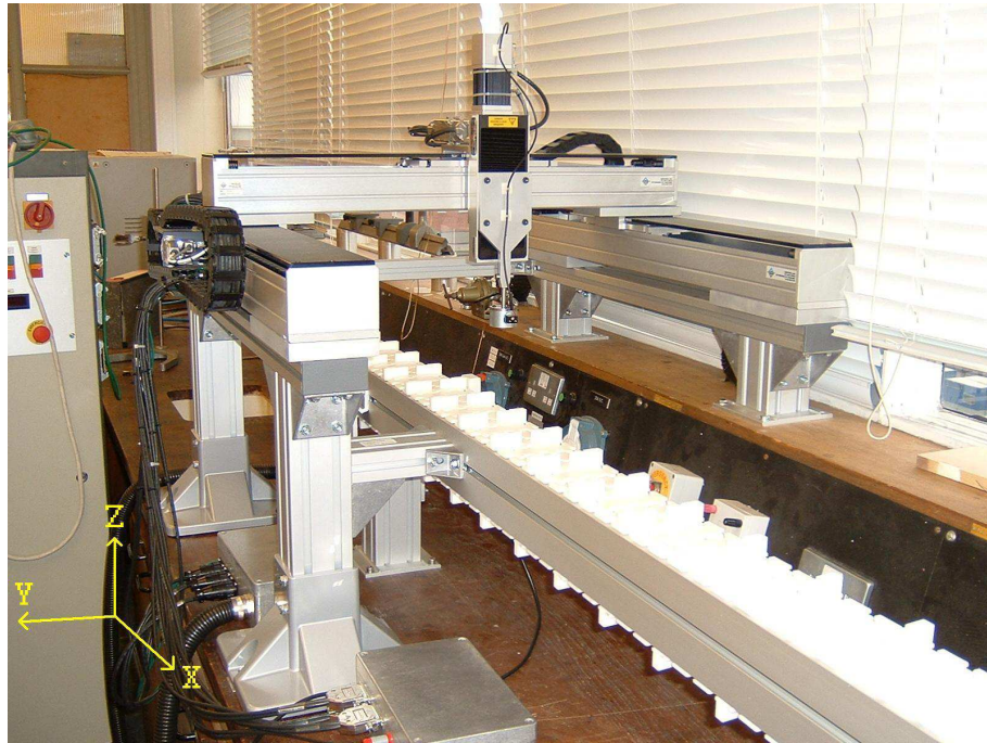
FIGURE 3.1: Gantry robot test facility with the axes marked.
