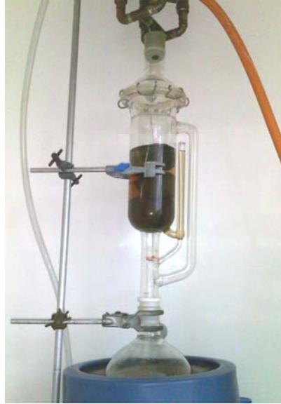
Figure 3.8. A picture showing samples that contain oil being washed in a Soxhlet reflux apparatus.
