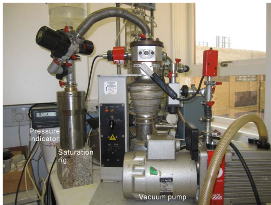
Figure 3.9. A picture showing samples being evacuated in the saturation rig.
