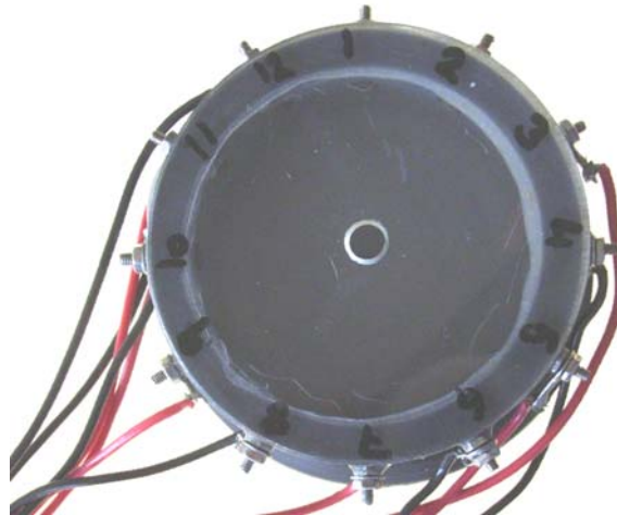
Figure 3.12. Brine calibration cell showing the configuration of the electrodes with exactly the same geometry as in the high pressure rig.
