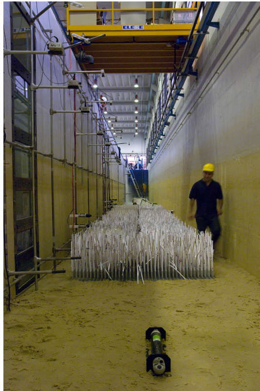
Figure 4.6 Overview of the patch and the instrument layout within the CIEM flume (looking towards the wave paddle). Wave gauges and velocimeters are secured to the sidewall.
