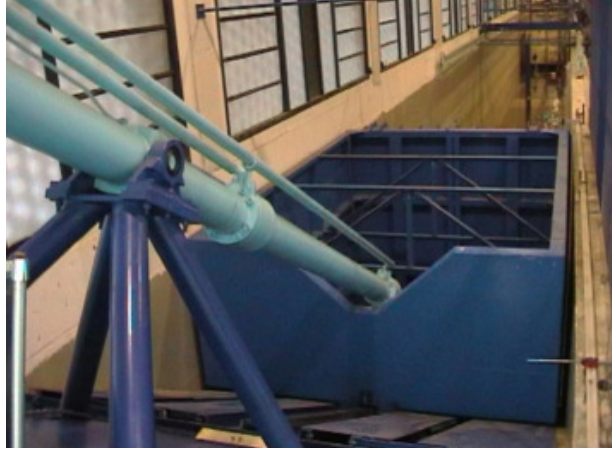
Figure 4.1 The CIEM wave generator (Photo courtesy LIM/UPC)
