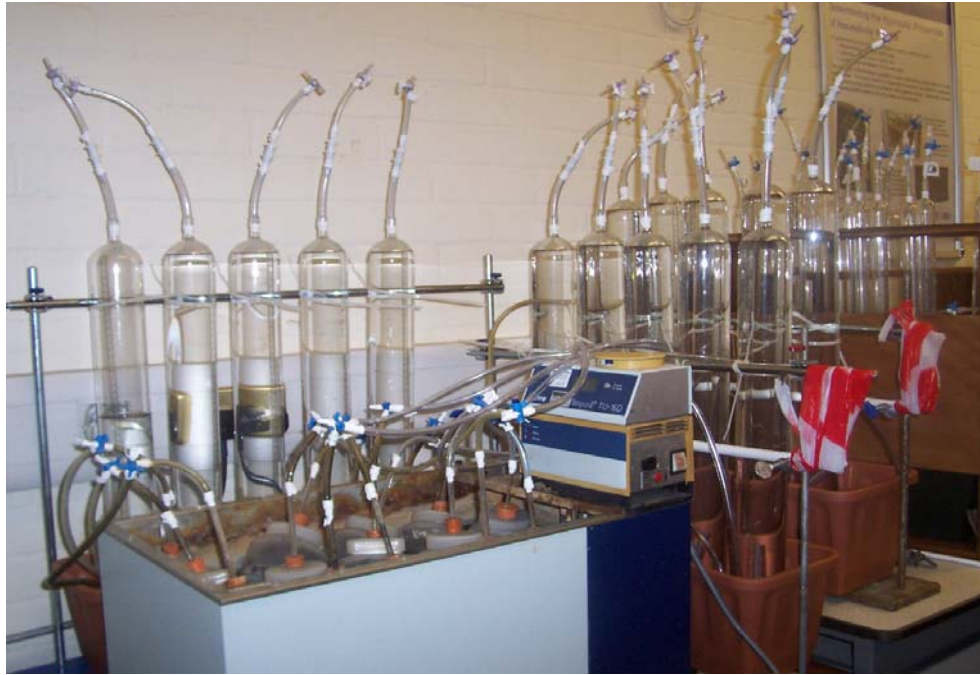
Figure 3.2 BMP test assay apparatus
