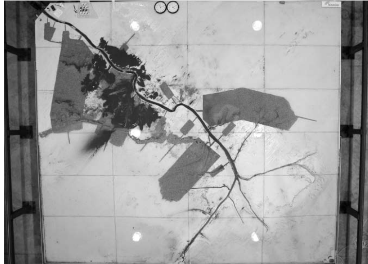
Figure 2.2: Overview of the small scale hydraulic model of the lower Mississippi river and delta, after Willson (2009).
