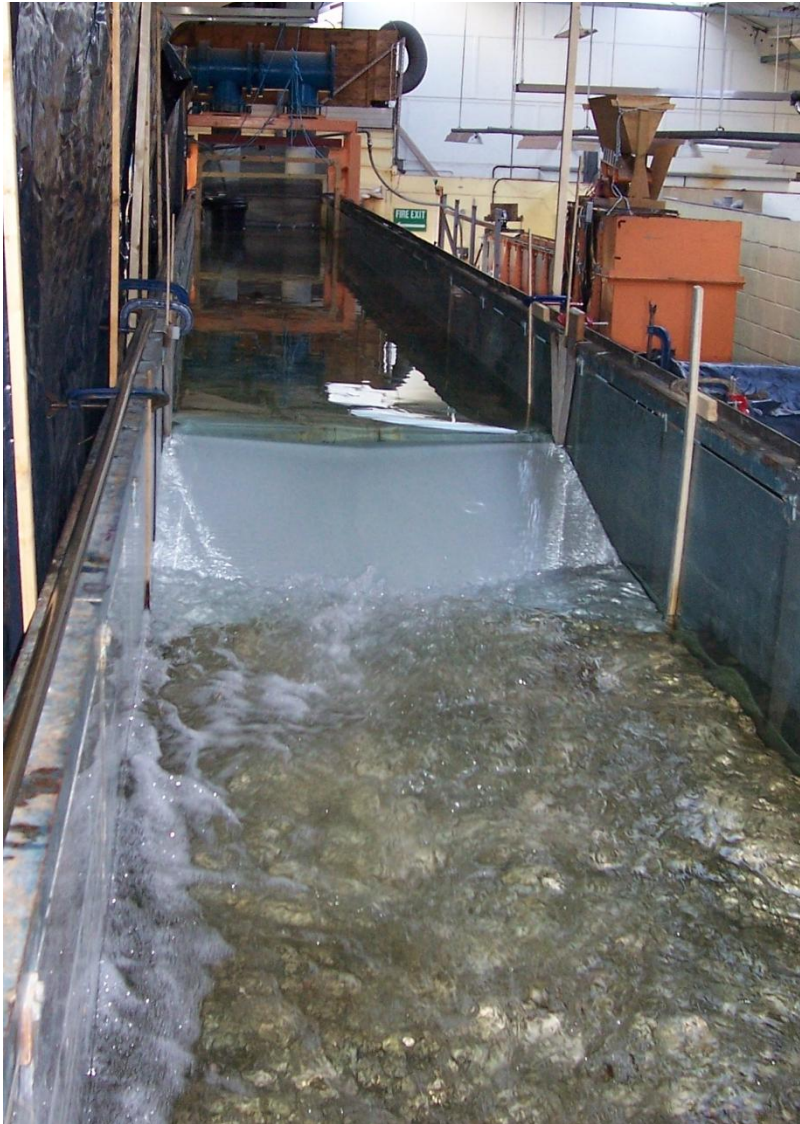
Plate 3.2 Chilworth flume facility retrofitted with a model flat-v gauging weir.
