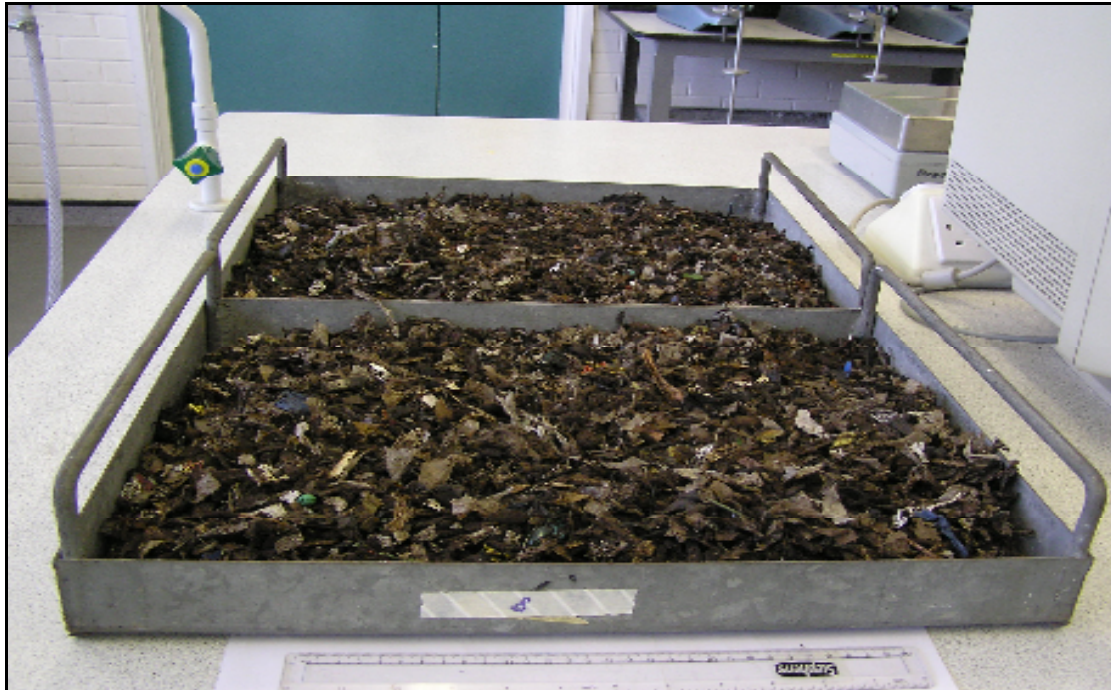
Figure 3.2: MBT waste sample as received from White's Pit waste processing plant (UK MBT waste)
