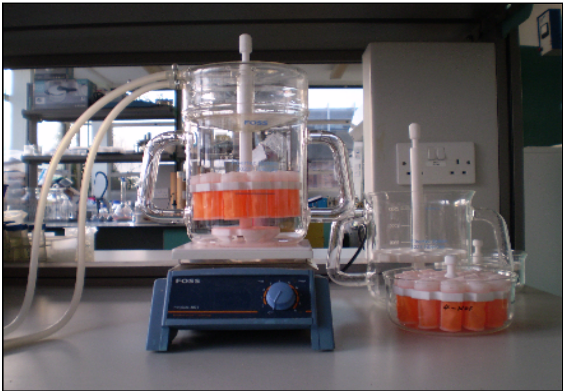
Figure 3.5: Foss Analytical FibreCap system for fibre analysis
