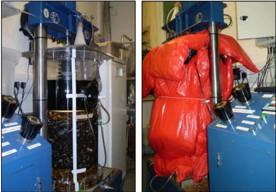
Figure 3.9: Consolidating anaerobic reactors, CAR1 and CAR2
