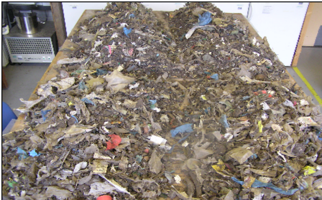
Figure 3.2: MBT waste sample as received from White's Pit waste processing plant (UK MBT waste)
