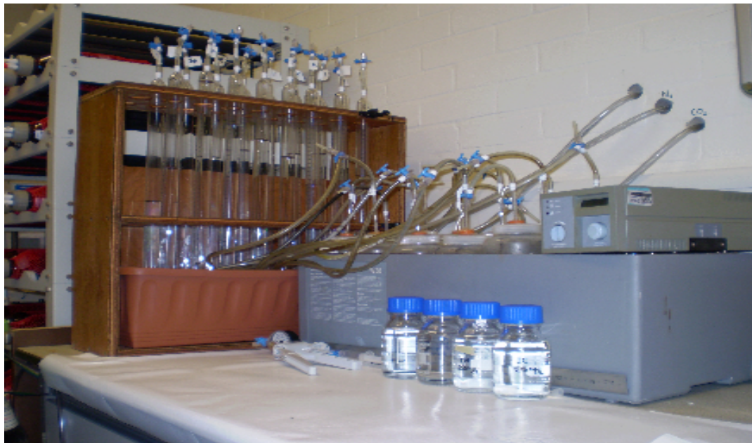
Figure 3.7: A schematic view and set up of biochemical methane potential test reactors
