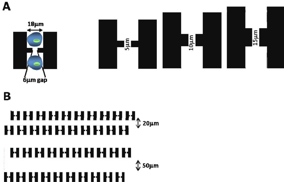
Figure 50 Dimensions of the different designed traps. *A*: Each trap has two hollows of  $18\mu\text{m}^2$ ,  $6\mu\text{m}$  gap of separation between the hollows. Drawn in blue are trapped cells. Three different distances between the 2 hollows were also tested:  $5\mu\text{m}$ ,  $10\mu\text{m}$  and  $15\mu\text{m}$ . *B*: Two different distances between the trap rows were also tested:  $20\mu\text{m}$  and  $50\mu\text{m}$ .
