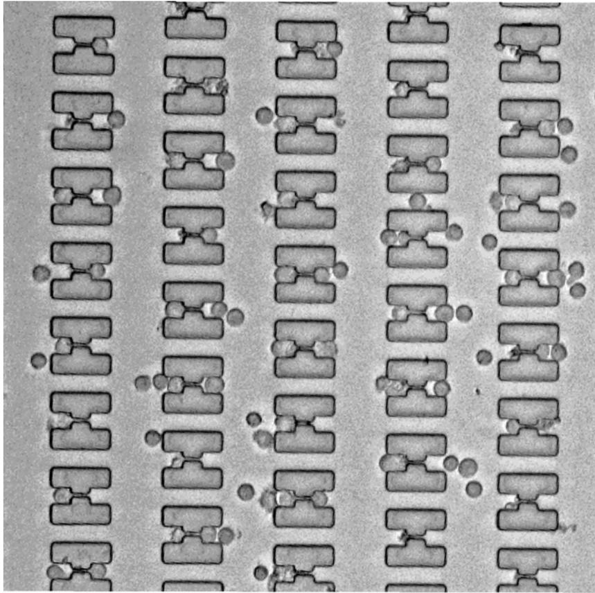
Figure 59 Loading efficiency of the devices. An example of one of the devices with cells loaded in both sides of the traps is shown. Efficiency (traps with both sides containing one cell) was estimated in 60% approximately.
