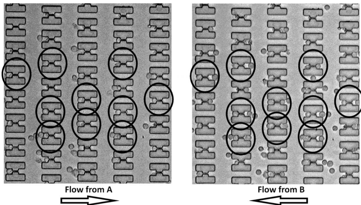
Figure 57 Flow workout of the device in two steps. A and B correspond to terminology used in Fig.56. Left picture shows the flow in of cells from channel A; channel B served as outlet. Right picture shows the filling of the device from channel B and thus, channel A served as outlet.
