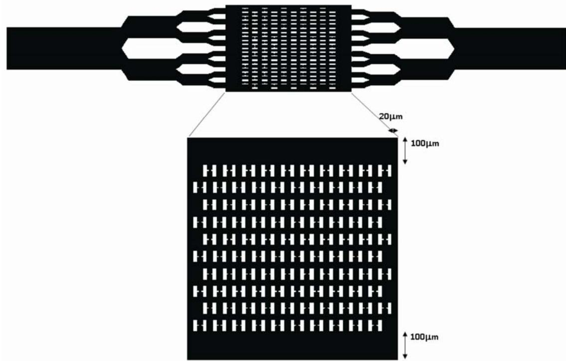
Figure 49 General view of the device. Separation distances between the rows of traps and the edge of the chamber are shown.
