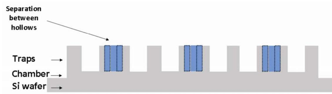
Figure 53 Section of the device showing the etched silicon wafer. Rows of traps were not parallel (see Fig. 50B) and this is indicated by the dotted lines. This patterned mold was used afterwards for PDMS molding and device making.
