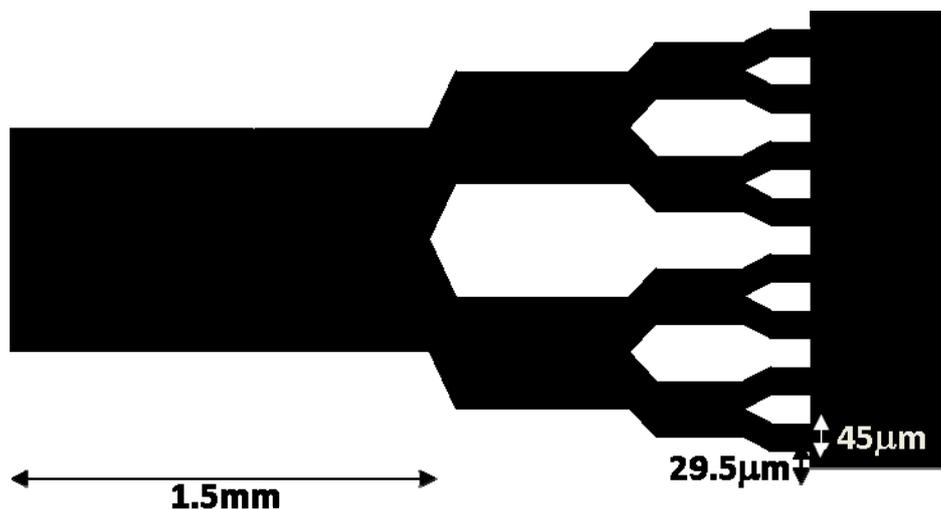
Figure 51 Schematic representation of the pipes design. The distance between the pipes and edges of the chamber was 29.5  $\mu\text{m}$  and the width of the pipes was 45 $\mu\text{m}$ . The length of the main branch was 1.5mm.
