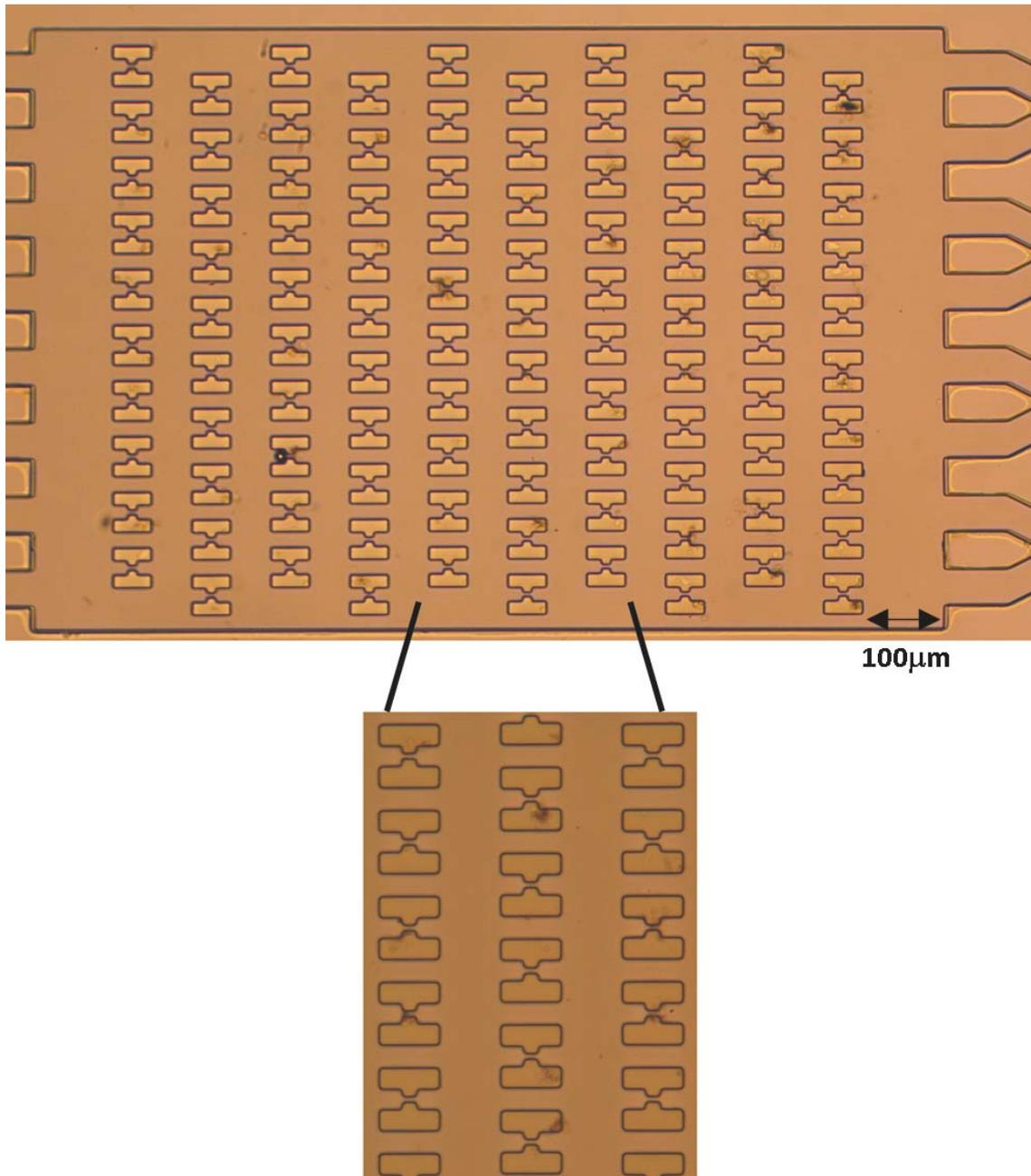
Figure 55 Picture of one of the devices in PDMS under the microscope. A zoom of a device is shown. The device shown corresponds to the design of 5 $\mu$ m gap and 50 $\mu$ m of separation between rows.
