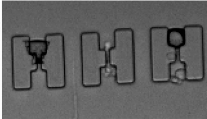
**Figure 58 Bubbles in microfluidic devices. A set of traps is shown; from left to right: a cell trapped (upper side), empty trap (with cell debris) and an air bubble with a disrupted cell (upper and lower sides, respectively).**
