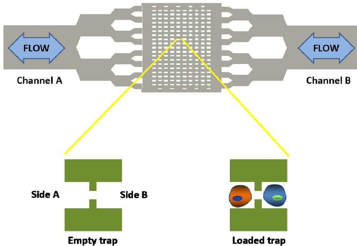
Figure 56 Flow representation in the devices. The chamber was filled first from the channel of one side and then from the one on the other side, represented as "A" and "B". These channels were alternatively used as inlet and outlet.
