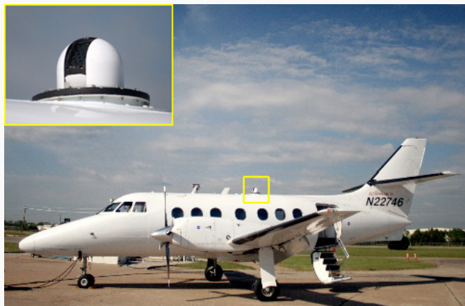
Jetstream-31 With NASA 14-Channel AATS (Ames Airborne Tracking Sunphotometer), ARM Climate Research Facility
