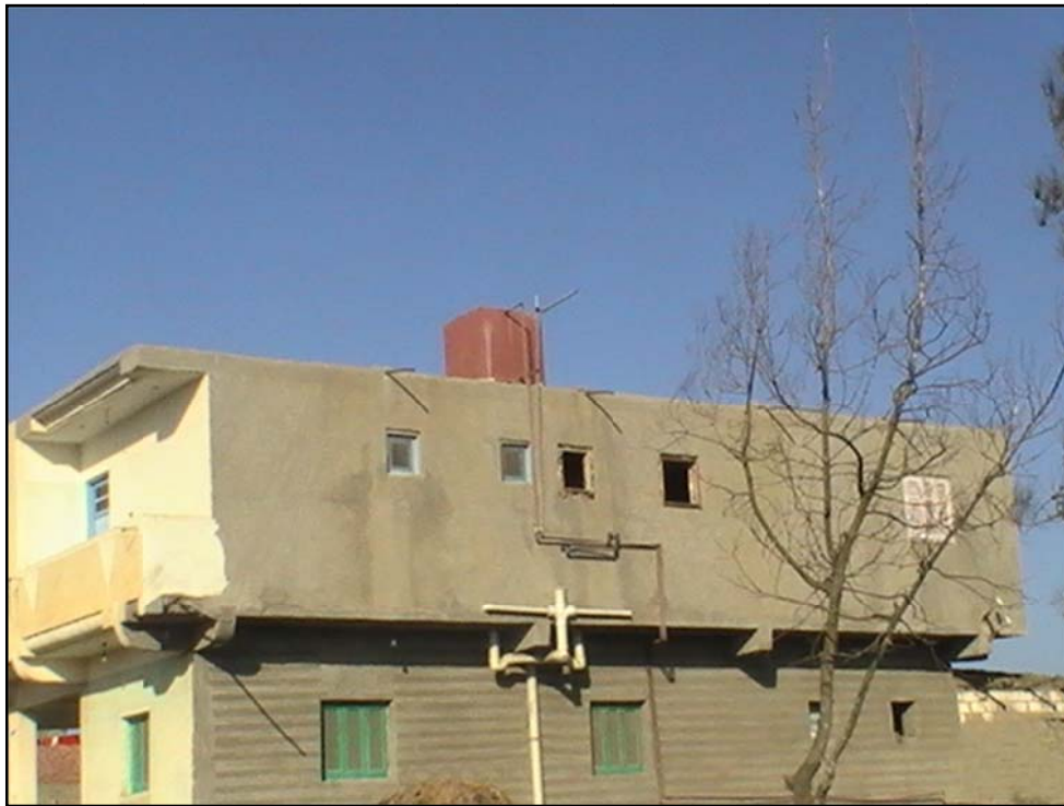
Figure 3.12 Picture illustrates a roof tank for storing drinking water used as a solution against water interruption
