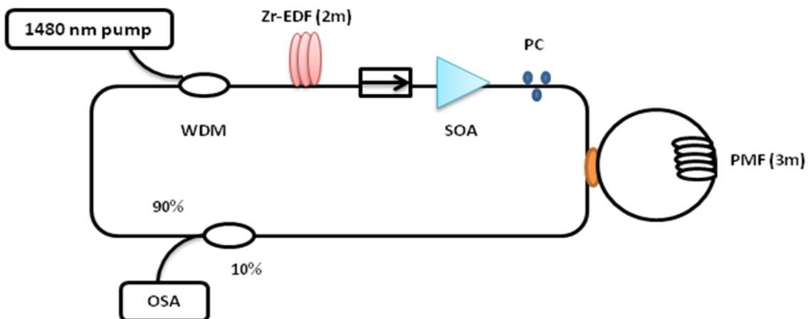
Fig. 1 (b). Ring cavity configuration.
