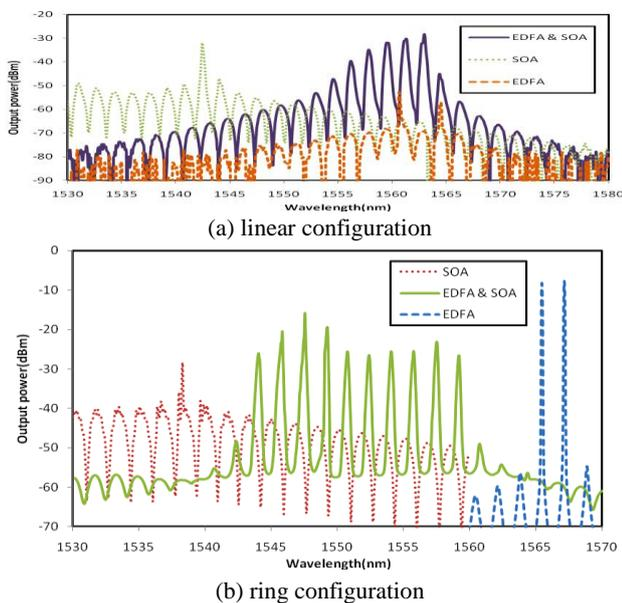
Fig. 2. Multi-wavelength optical amplifiers with an SOA and EDZF (a) linear (b) ring configurations.
