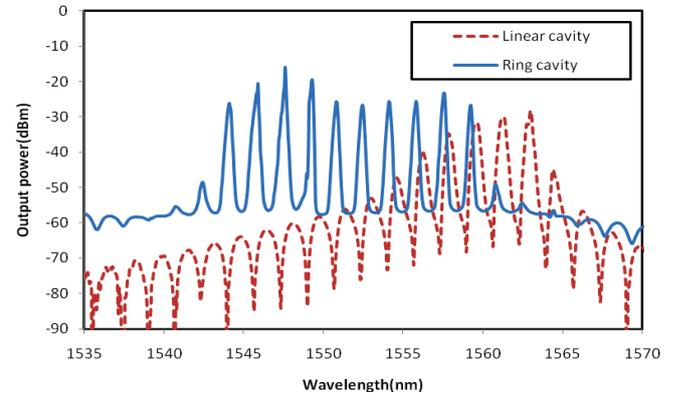
Fig. 3. Comparison of the output spectrum between two hybrid EDZF/SOA amplifiers configured with ring and linear cavity.
