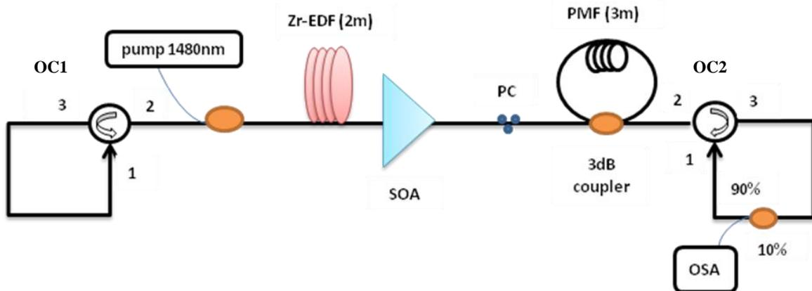
Fig. 1(a). Linear cavity configuration.
