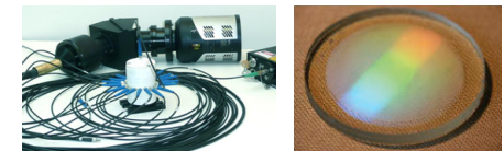
Figure 6. PPO instrument multichannel spectrometer (left) and VPH transmission grating. Spectrometer (SPEC)
