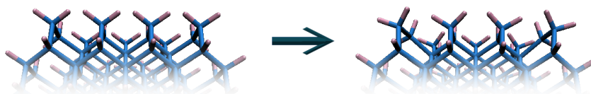
Figure 4.11: Schematic representation of symmetric hydrogens (before geometry optimisation) and “canted” hydrogens (after geometry optimisation) located on a part of the surface of the (1\times 1) reconstructed \text{Si}_{766}\text{H}_{462} nanorod
