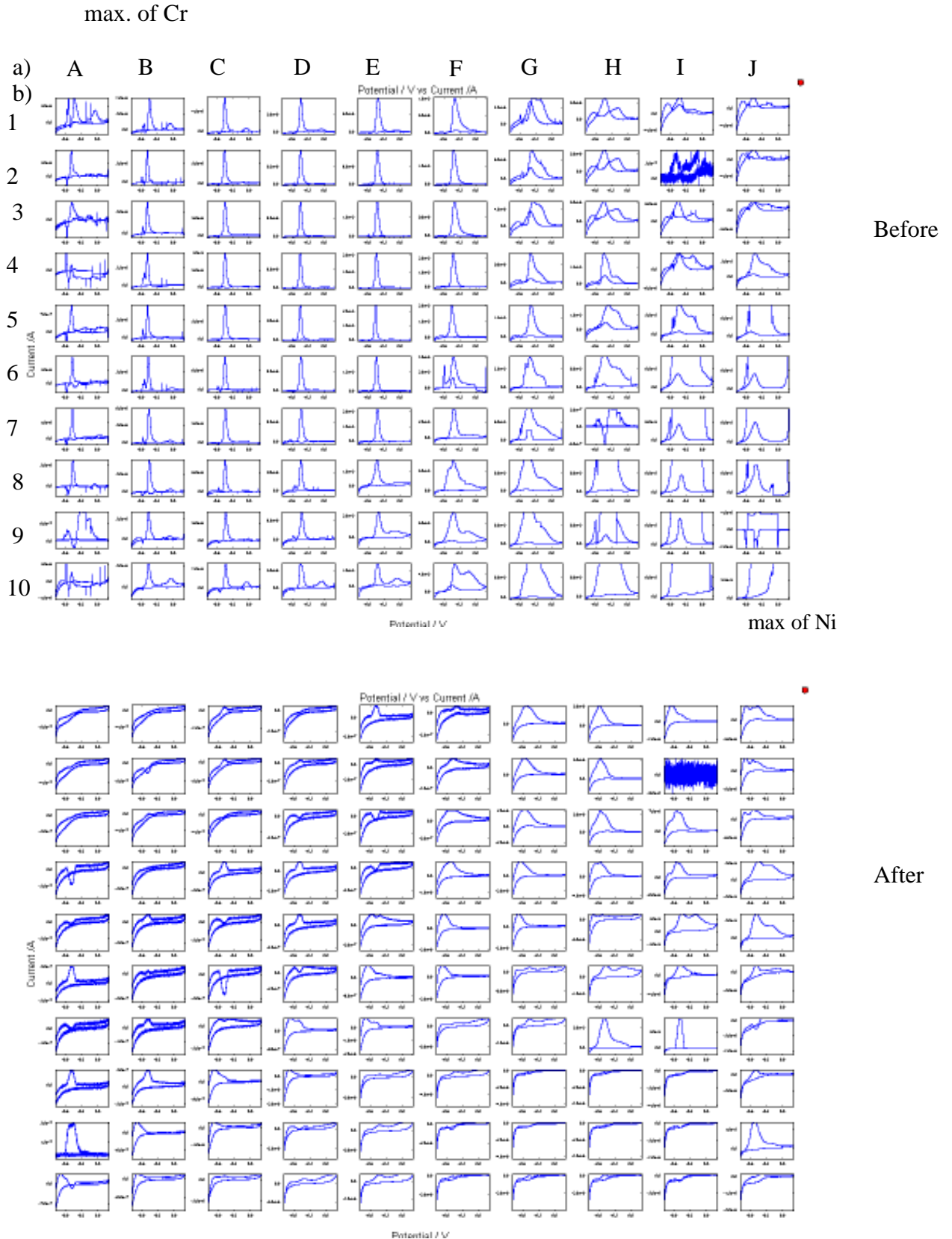
Figure 5.2.2.2 Cyclic voltammograms of 100-electrodes array Ni-Cr alloys of heat treated sample in phosphoric acid pH 2 at 323 K for a) first scan, b) scan after step experiment. Potential scan rate 20 \text{ mV s}^{-1} .
