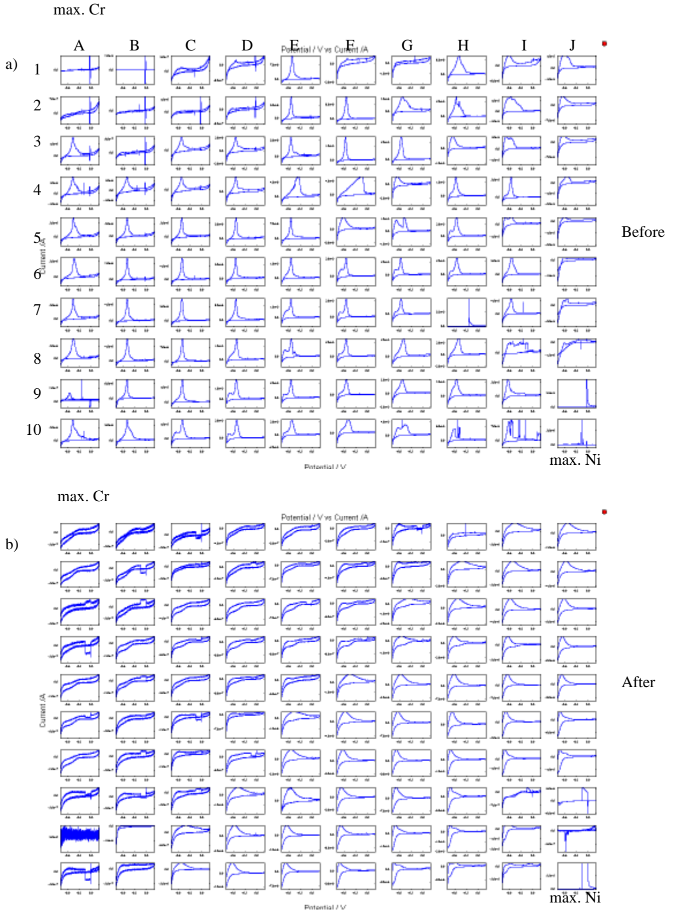
Figure 5.2.1.2 Cyclic voltammograms of 100-electrodes array Ni-Cr alloys in phosphoric acid pH 2 at 323 K for a) first scan, b) scan after step experiment. Potential scan rate 20 \text{mV s}^{-1} , potential range: - 800 mV to + 200 mV vs. \text{Hg}/\text{Hg}_2\text{SO}_4 .
