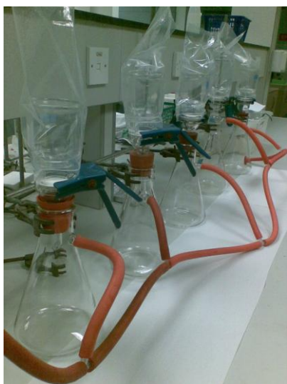
Figure 3 Vacuum filtration apparatus used in this study.
