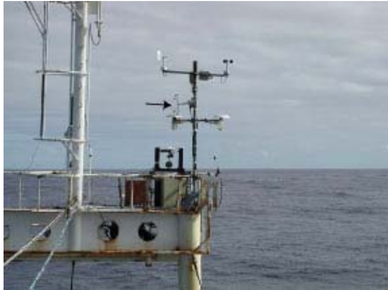
Figure 5.3 The foremast of the RRS Charles Darwin , showing the HS sonic anemometer (indicated by the arrow) on the starboard side of the platform.
