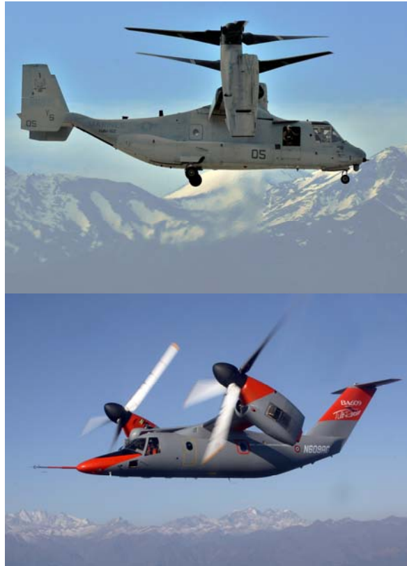
Figure 3.66: Tilt-Rotor aircraft provide higher speed and range whilst maintaining the ability to take off and land vertically. Top: The V-22 Osprey military tilt-rotor has seen operational deployment, photo courtesy of the United States Department of Defence. Bottom: The BA609 civil tilt-rotor is undergoing certification, photo courtesy of AgustaWestland.
