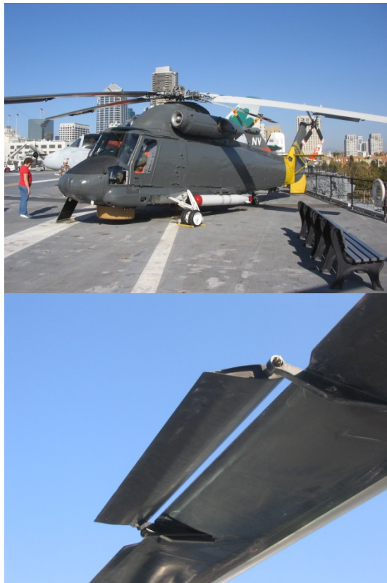
Figure 1.15: The Kaman H-2 Seasprite helicopter and a close up of its servo-flap primary control system. Photographed by the author at the USS Midway Aircraft Carrier Museum, 2009.
