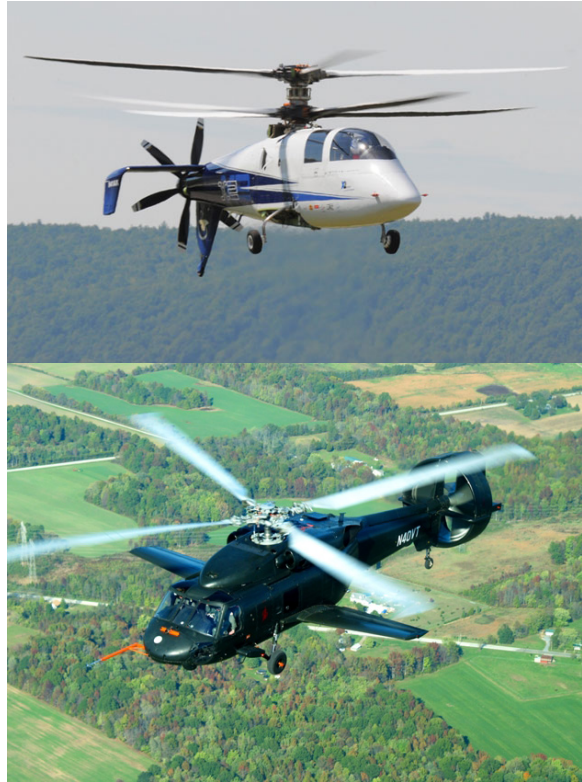
Figure 3.67: Recent technology demonstrator aircraft for higher-speed helicopters. Top: The Sikorsky X2 demonstrating the Advancing Blade Concept, photo courtesy of Sikorsky. Bottom: The Piasecki X-49A Speedhawk demonstrating the Vectored Thrust Ducted Propeller concept.
