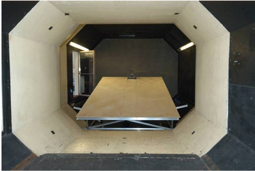
Figure 4.38: Image of the rotor model mounted at position A on the ramp in the wind tunnel. Note that the flow direction is towards the observer such that the ramp provides a leeward-facing slope. Image courtesy of Dr S. Newman.
