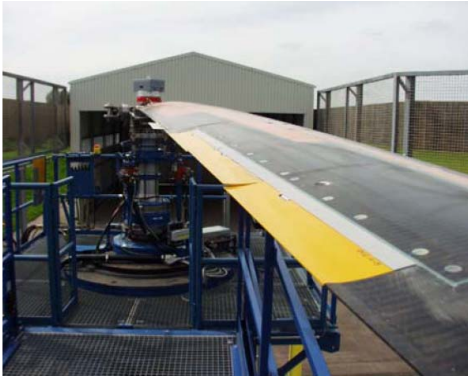
Figure 1.28: Image of the Eurocopter Deutschland active flap equipped blade during whirl tower testing. Image reproduced from Roth et al (2006).
