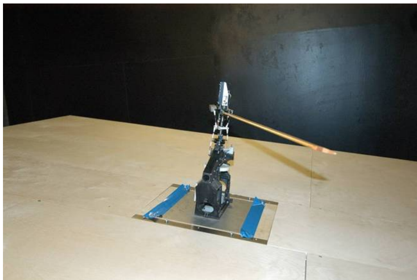
Figure 4.39: Close-up image of the single-blade teetering rotor model mounted at position B on the ramp. Image courtesy of Dr S. Newman.
