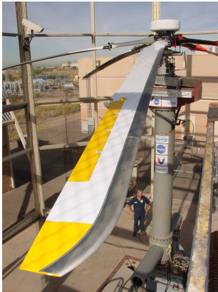
Figure 1.26: The Boeing Smart Material Actuated Rotor Technology (SMART) active flap equipped rotor during whirl tower testing. Image reproduced from Straub et al (2004).
