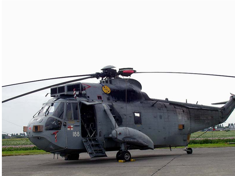
Figure 4.27: Image of a Sea King Helicopter with centrisep
