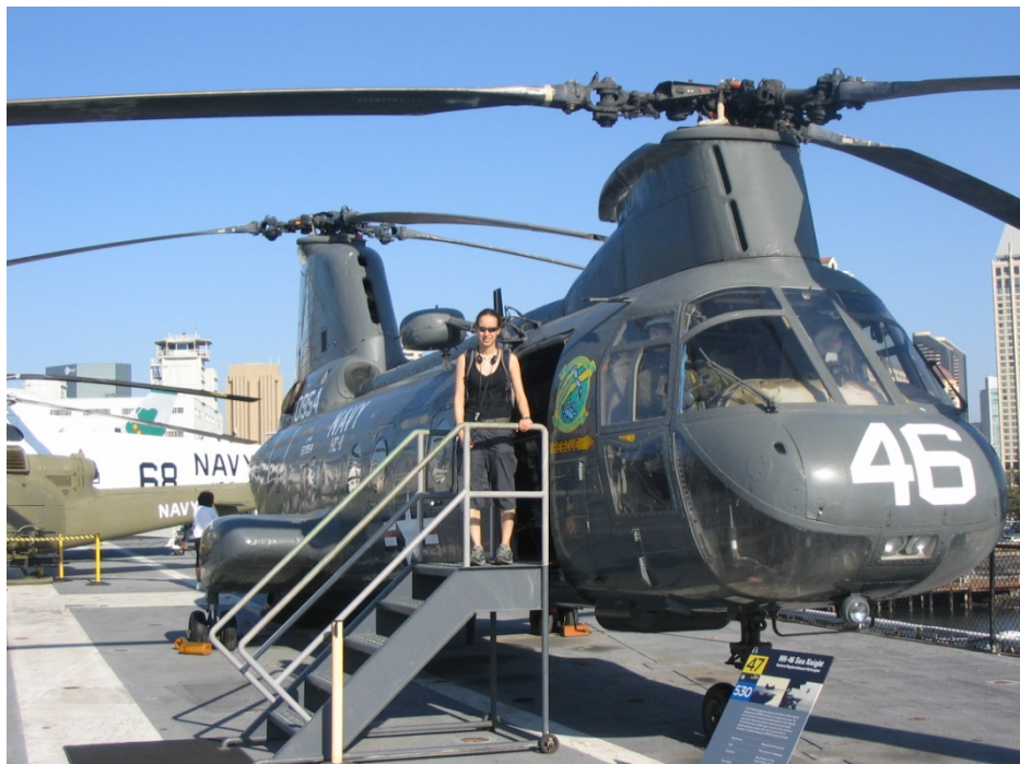
Figure 4.7: The CH-46 Sea Knight helicopter. Note the blade flexibility evident in the rear rotor and the tandem rotor layout with the transmission ‘tunnel’ between the rotor pylons. Photographed by the author at the USS Midway Aircraft Carrier Museum, 2009.
