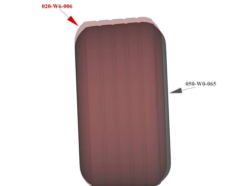
Figure 2.3: Comparison of the two experimental wheels used. The wheel used for pressure measurements is labelled 020-W6-006 and the wheel used for PIV and forces is labelled 050-W0-065.
