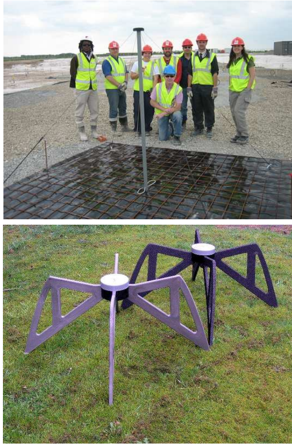
Figure 1.5: Top panel: The first Low Band Antenna (LBA) to be constructed at the LOFAR UK Chilbolton station. The antenna consists of a low noise amplifier mounted on a piece of tubing, which is secured via the XX and YY polarised dipole wires to a reflective ground plane (credit: LOFAR UK). Bottom panel: Two High Band Antennas (HBA) which are typically deployed in 4 \times 4 tiles within a protective casing (credit: Astron).
