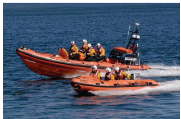
Figure 1: In the foreground shows the IB1 and in the background shows the Atlantic 85 RIB [1]
