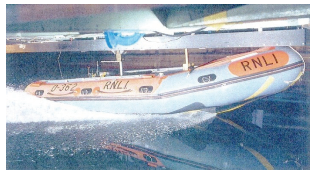
Figure 9: Spray generation of an EA16 at 19.4 knots [12]
