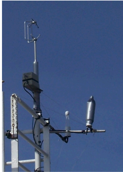
Figure 2.6. Components of the AutoFlux turbulent flux system installed on the Polarfront 's foremast. The instrument configuration shown here was in place from January 2008 to December 2009 (Table 2.5). The photograph was taken from the aft-starboard side of the ship, looking towards the fore of the ship. The right-hand IRGA is shrouded.
