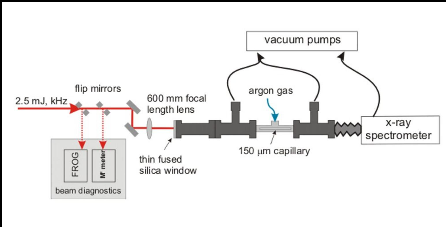
Harmonic generation in low-pressure argon gas in a hollow capillary waveguide
