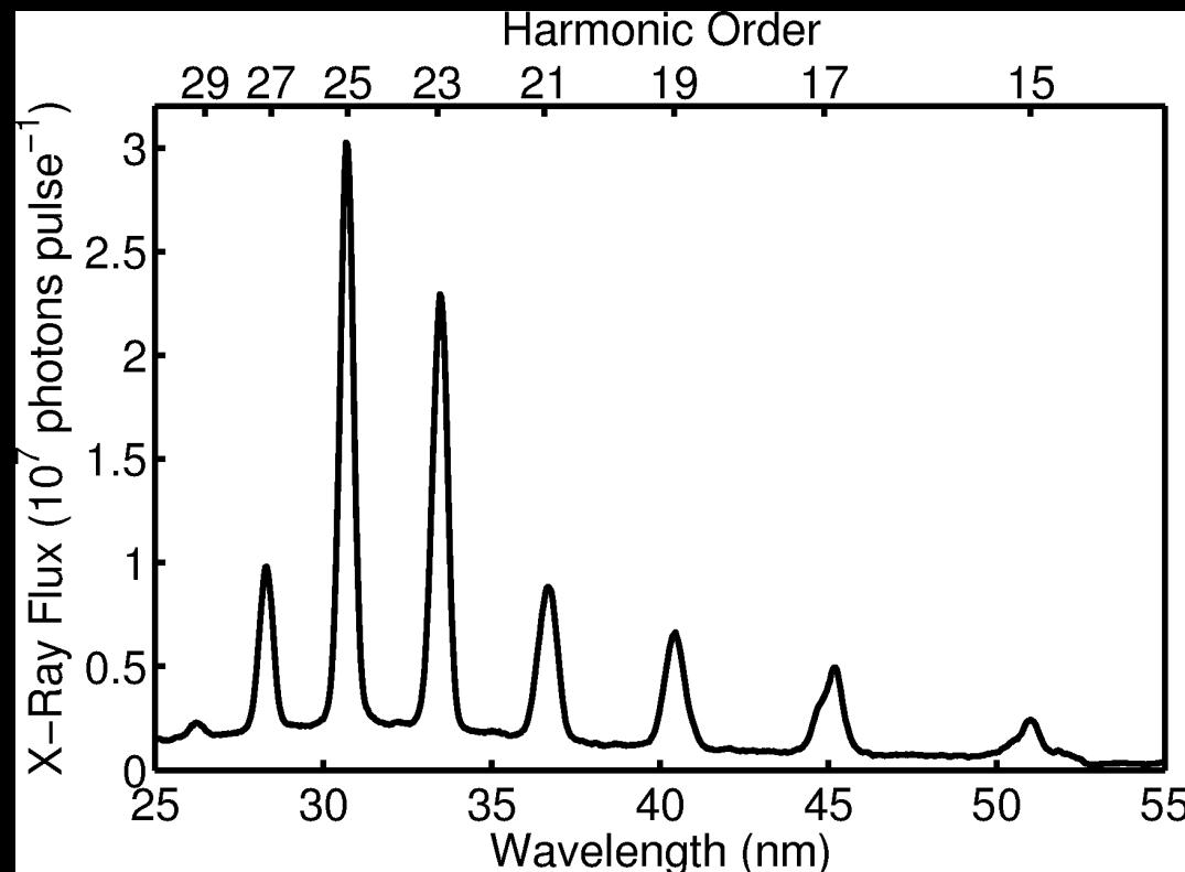
High harmonic spectrum measured with grazing incidence spectrometer using a multi-channel plate detector. A 200 nm Al foil is used to filter laser. Optics Letters, in press.
