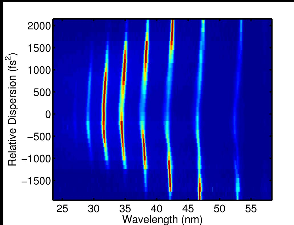
Optimisation of the X-ray harmonic spectrum by pulse shaping
