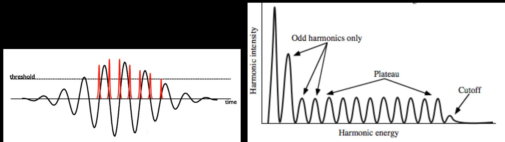
Ionization and recollision repeats every half-cycle and produce a comb of frequencies up to the cutoff
