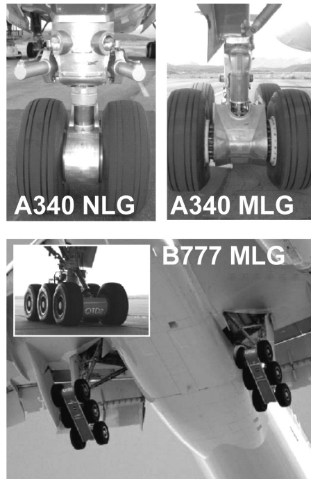
Figure 2.12: Examples of landing gear add-on fairings [1].
