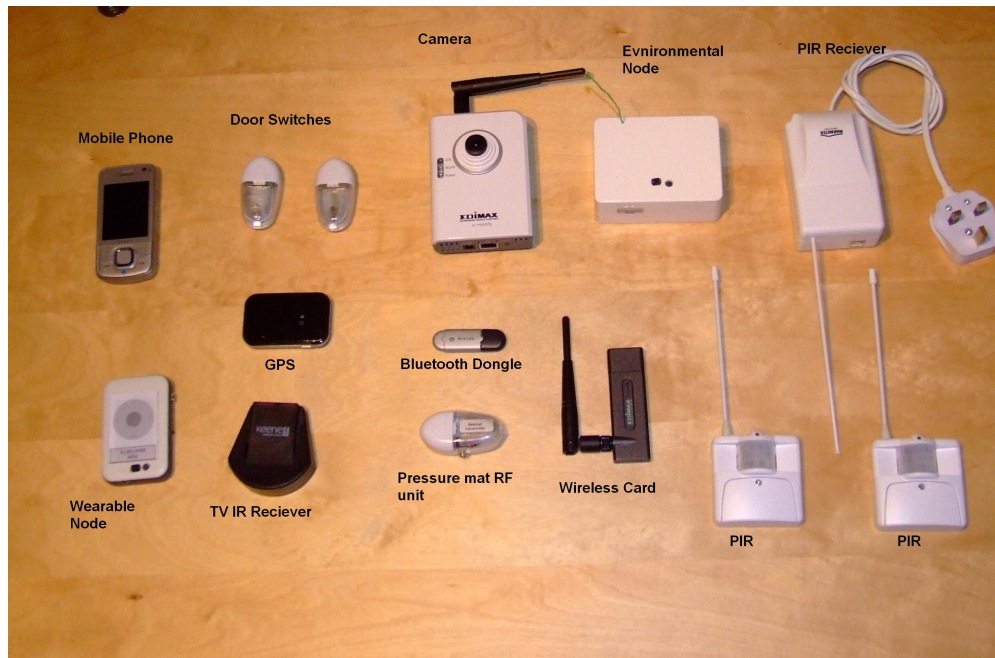
FIGURE 3.2: The sensors for the PAM self-management system that were used in the technical trial. Both sub-systems are shown; the wearable sub-system, comprising the phone, wearable node and GPS, and the environmental sub-system, comprising everything else.
