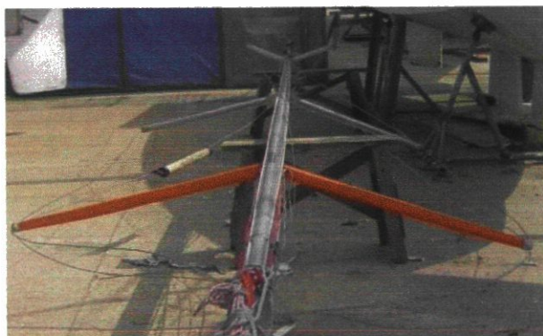
fig. 2.2 – two swept spreaders plus jumpers
