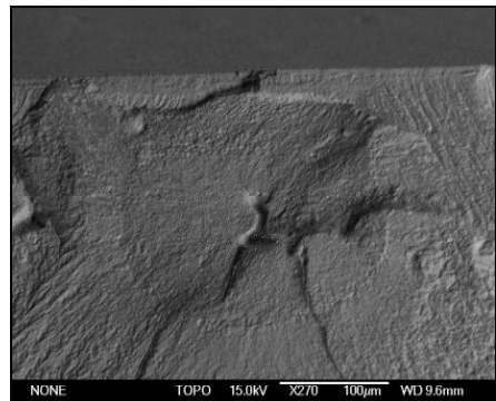
Figure 3 Subsurface initiation viewed using BEI (topographical)
