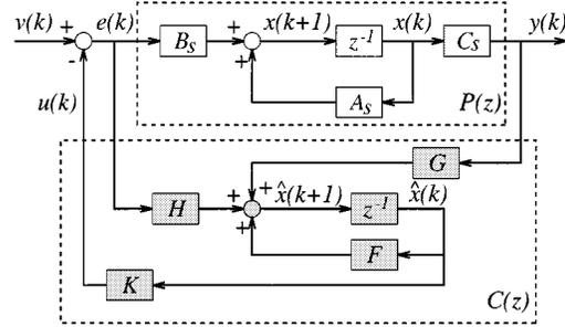
Fig. 1. Block diagram of the closed-loop system with state-estimate feedback controller.
