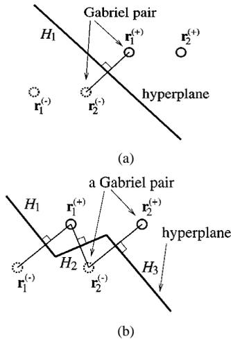
Fig. 1. The two typical cases of the asymptotic Bayesian decision boundary for channel  $\mathbf{a} = [a_0 \ a_1]^T$ . The DFE structure is defined by  $m = 2$ ,  $d = 1$ , and  $n = 1$ .
