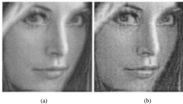
Fig. 9. Face portions of PC coded (coding bit = 1, quantizing step = 4) and post-improved images of "Lena." (a) PC coded (PSNR = 24.17 dB). (b) NNVM (PSNR gain = 2.87 dB).
