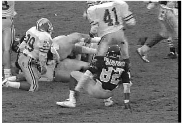
Figure 3. Frame 79 of "Football" sequence which illustrated minor decoding error at BER of 2 \cdot 10^{-4} after convolutional decoding. The PSNR degradation observed is approximately 2 dB. The sequence was coded using rate 7/8 convolutional codes and transmitted using QPSK modulation.
