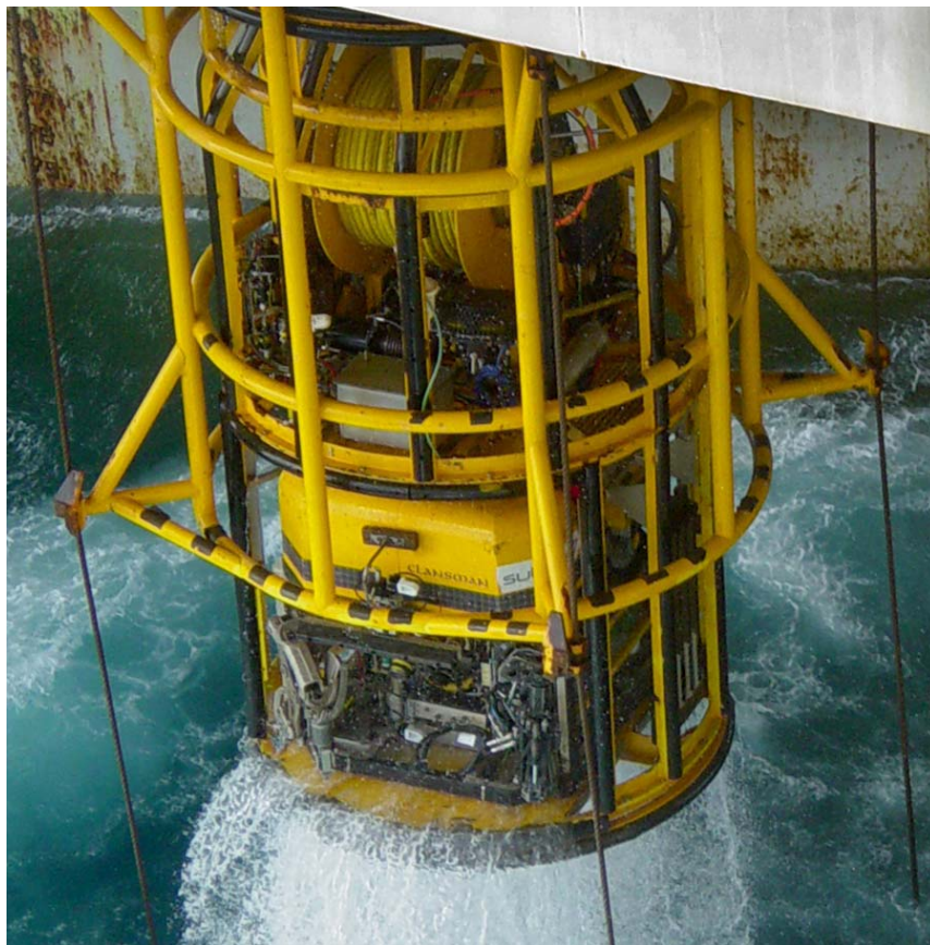
Figure 2.2: Clansman ROV returning to Jack Bates Rig. ROV is contained within yellow ‘garage’ used for transport to and from the surface. Note the Tether Management System (TMS) above the ROV. The entire inner yellow cage is lowered to around 50m from the seabed and the ROV launched from the garage using the 250m long yellow tether (coiled on the TMS) to move around.
