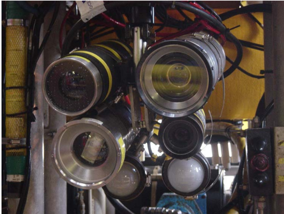
Figure 2.3: Camera package on Clansman 2. (Top Left) SIT system (Top Right) OE14-208 Stills, (Bottom Left) Still Flash Unit, (Bottom Right) Pan – Tilt Colour Video.
