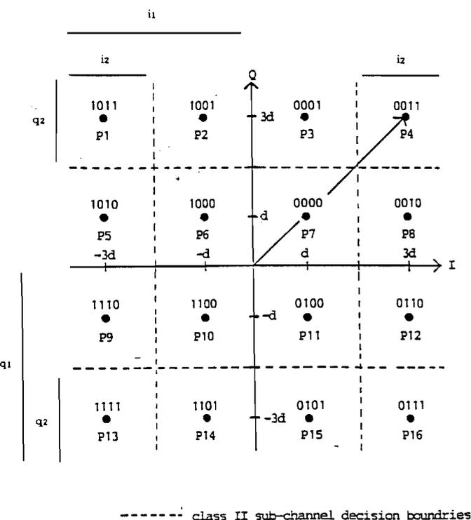
Fig.1: 16-level QAM constellation
