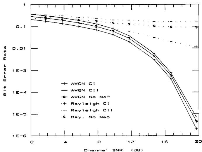
Fig.2: CI and CII BER variation vs. channel SNR
