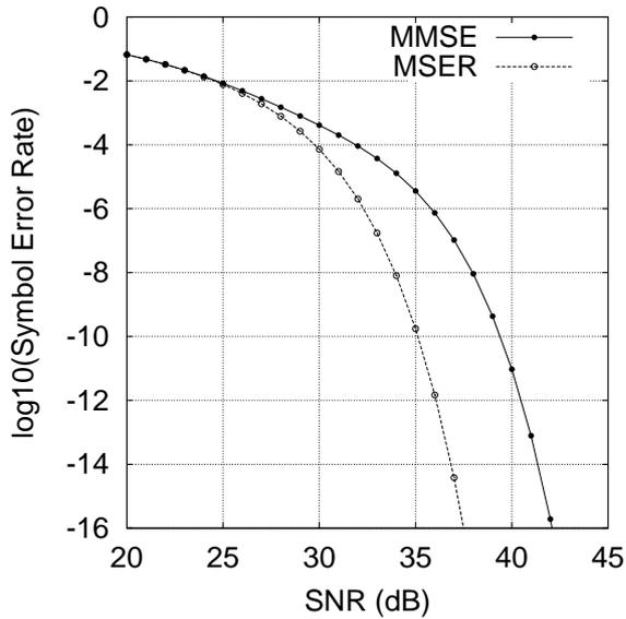
Fig. 2. Lower-bound symbol error rate comparison for Example 2, assuming correct symbols being faded back.
