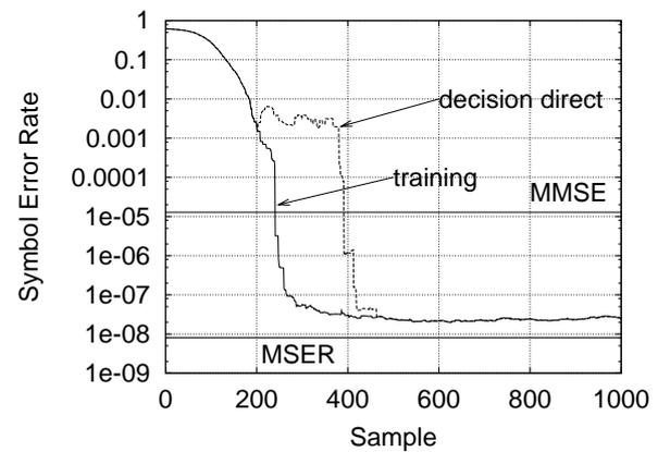
Fig. 4. Learning curves of the LSER for Example 2 with SNR= 34 dB, averaged over 100 runs. Initial  $\mathbf{w} = [-0.01 \ 0.01 \ 0.01]^T$ . Dashed curve: after 200-sample training, switched to decision-directed adaptation with  $\hat{s}(k-d)$  substituting  $s(k-d)$ .
