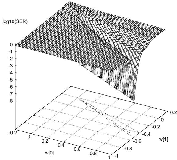
Fig. 1. The SER surface for Example 1 with SNR= 35 dB. The MMSE solution  $\mathbf{w}_{\text{MMSE}} = [0.929 \ -0.371]^T$ , which has been normalized, with  $\log_{10} P_E(\mathbf{w}_{\text{MMSE}}) = -2.7593$ . The MSER solution  $\mathbf{w}_{\text{MSER}} = \alpha[0.896 \ -0.445]^T$ ,  $\alpha > 0$ , with  $\log_{10} P_E(\mathbf{w}_{\text{MSER}}) = -7.1566$ .
