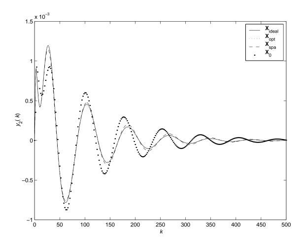
Figure 3: Comparison of second-input second-output unit impulse response of the infinite-precision controller implementation  $\mathbf{X}_{ideal}$  with those of the 24-bit implemented controller realizations  $\mathbf{X}_0$ ,  $\mathbf{X}_{opt}$  and  $\mathbf{X}_{spa}$  for Example 2.
