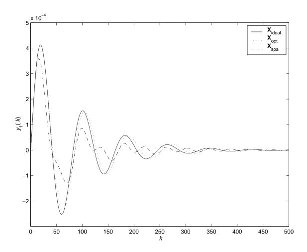
Figure 2: Comparison of first-input first-output unit impulse response of the infinite-precision controller implementation  $\mathbf{X}_{ideal}$  with those of the 20-bit implemented controller realizations  $\mathbf{X}_{opt}$  and  $\mathbf{X}_{spa}$  for Example 2. The 20-bit implemented  $\mathbf{X}_0$  is unstable.
