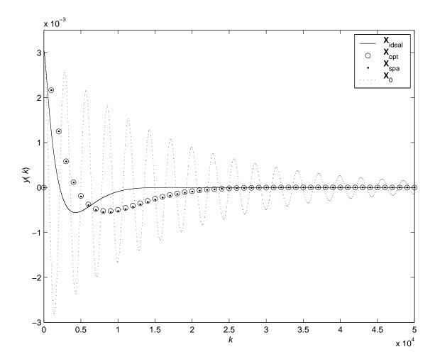
Figure 1: Comparison of unit impulse response of the infinite-precision controller implementation  $\mathbf{X}_{ideal}$  with those of the three 16-bit implemented controller realizations  $\mathbf{X}_{0}$ ,  $\mathbf{X}_{opt}$  and  $\mathbf{X}_{spa}$  for Example 1.
