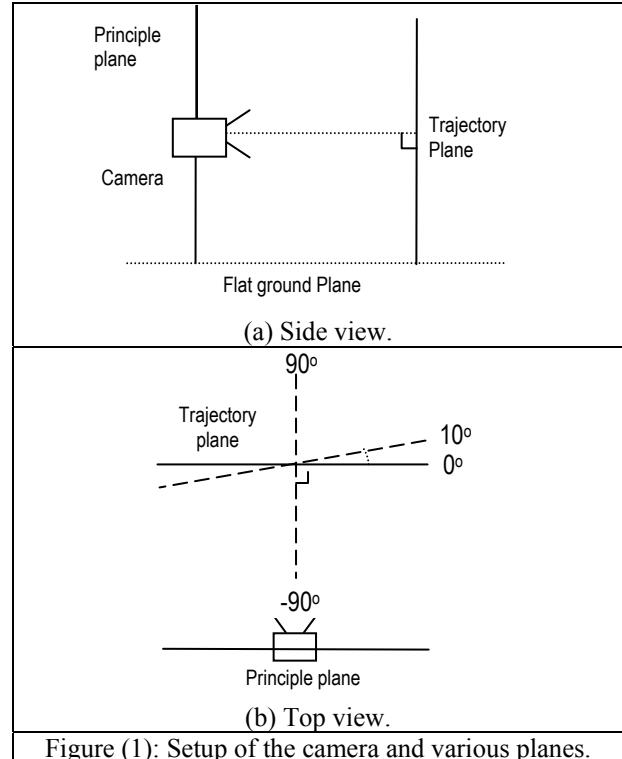
Figure (1): Setup of the camera and various planes.
