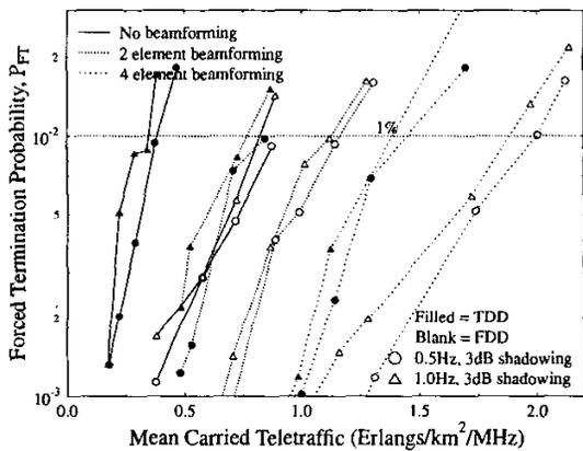
Figure 5: Call dropping probability versus mean carried traffic of the UTRA-like TDD/CDMA based cellular network both with as well as without beamforming and with shadowing for SF=16.
