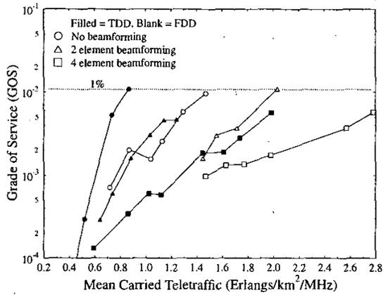
Figure 4: Grade-Of-Service (GOS) versus mean carried traffic of the UTRA-like TDD/CDMA based cellular network both with as well as without beamforming and without shadowing for SF=16.
