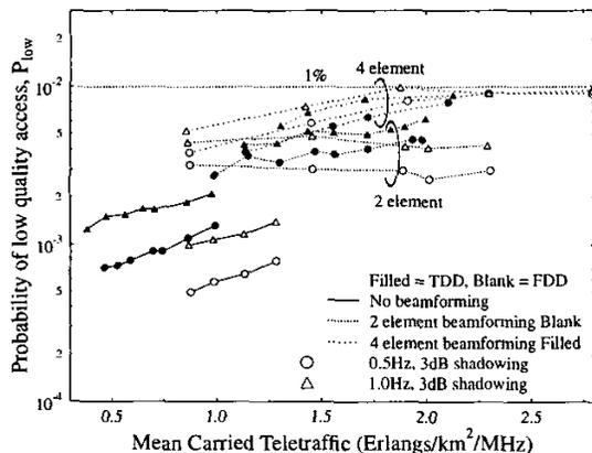
Figure 8: Probability of low quality access versus mean carried traffic of the UTRA TDD/CDMA based cellular network both **with and without beamforming in conjunction with AQAM as well as with shadowing having a standard deviation of 3dB for SF=16.**
