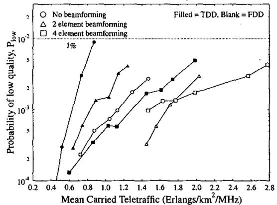
Figure 3: Probability of low quality access versus mean carried traffic of the UTRA-like TDD/CDMA based cellular network both with as well as without beamforming and without shadowing for SF=16.
