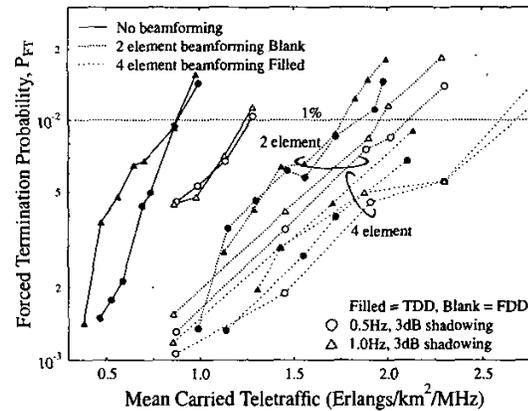
Figure 7: Call dropping probability versus mean carried traffic of the UTRA-like TDD/CDMA based cellular network both with and without beamforming in conjunction with AQAM as well as with shadowing having a standard deviation of 3 dB for SF=16.
