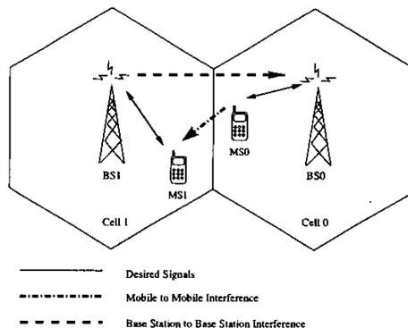
Figure 1: Inter-cell interference.
