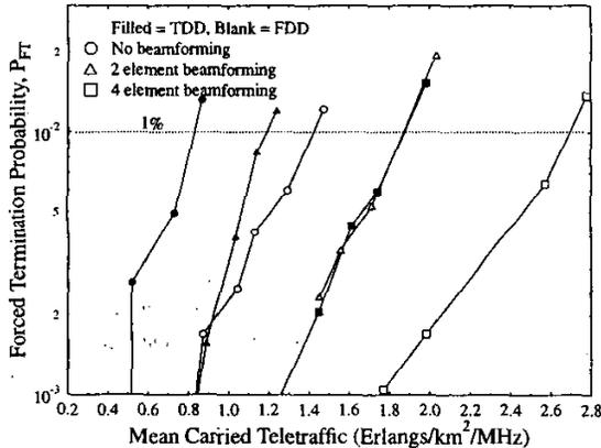
Figure 2: Call dropping probability versus mean carried traffic of the UTRA-like TDD/CDMA based cellular network of Table 1 both with as well as without beamforming and without shadowing for SF=16.
