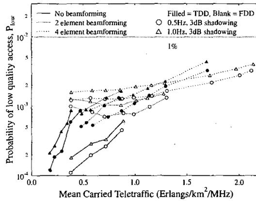
Figure 6: Probability of low quality access versus mean carried traffic of the UTRA-like TDD/CDMA based cellular network both with as well as without beamforming and with shadowing for SF=16.
