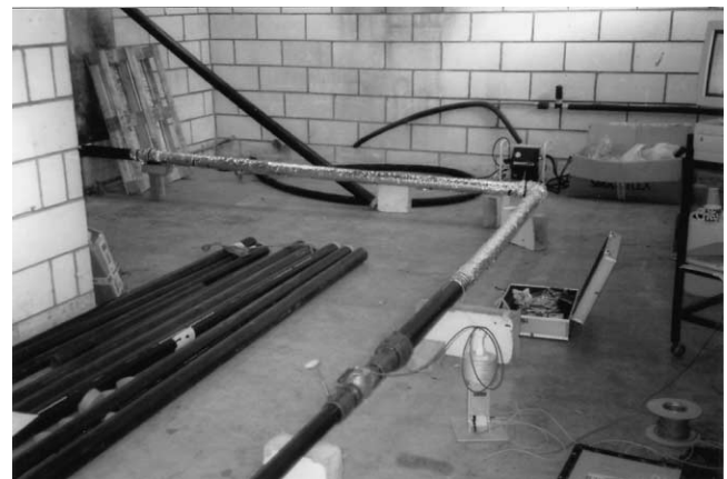
Fig. 3. Test pipeline for fuel-flow trials showing pipe, electro-fusion couplers and valve. The 90° elbow in this photograph is coupling number 9. Spare pipe sections can be seen on left.
