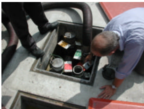
Plate 3. Measurement of electrostatic potential after filling.
