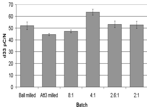
Fig 4: Average measured d<sub>33</sub> value for each powder combination.
