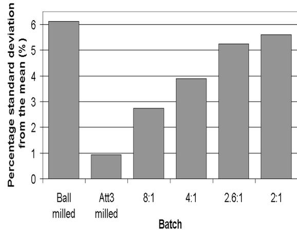
Fig 5: Percentage standard deviation for the measured d<sub>33</sub> value of each powder combination.
