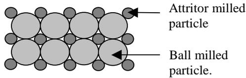
Fig 1: Ideal 2D model for particle distribution.
