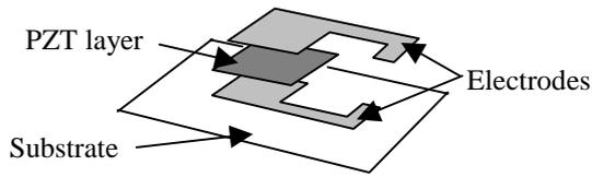
Fig 3: Capacitive structure for the piezoelectric device
