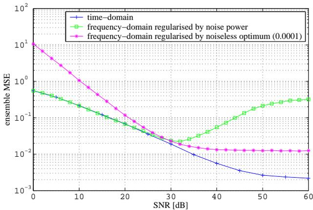
**Fig. 4.** MSE curves for  $z$ , time and frequency-domain inversion in a severely time-dispersive noisy environment with a non-minimum phase channel determinant.
