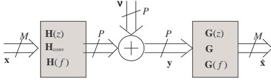
**Fig. 1.** Schematic of a known MIMO channel and a MIMO equaliser shown in three different domains.
