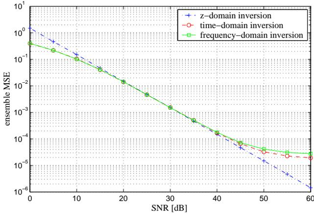
**Fig. 3.** MSE curves for  $z$ , time and frequency-domain inversion in a severely time-dispersive noisy environment with a minimum phase channel determinant.
