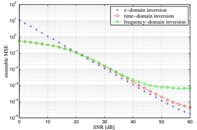
**Fig. 2.** MSE curves for  $z$ , time and frequency-domain inversion in a mildly time-dispersive noisy environment.
