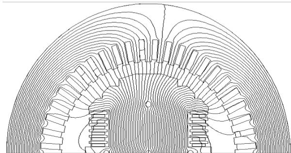
Figure 3 Flux lines in the proposed superconducting rotor at full load (showing one pole)
