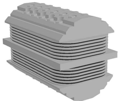
Figure 2 Construction of the rotor core and HTS coils.
