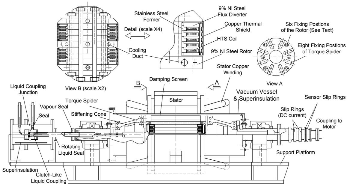
Figure 1 Sketch of the 100kVA HTS generator.
