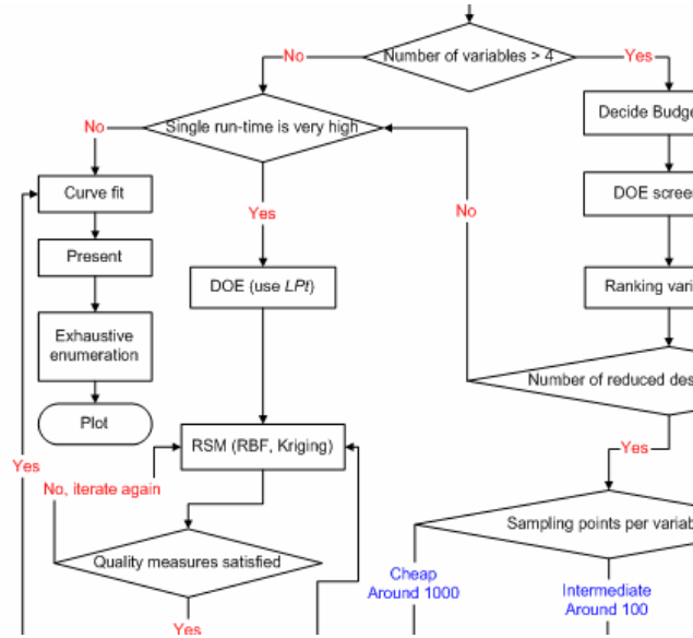
Fig. 3. Fragment of EDSO Design Process Flowchart
