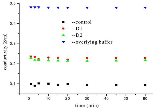
Fig. 8 Conductivity of the overlying buffer from the suspension used in Figs. 6 and 7 compared to that of dead cells (D1 and D2) and control buffer.
