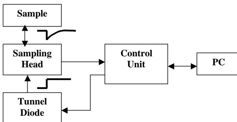
Fig. 2 Schematic diagram of TDS measurement.
