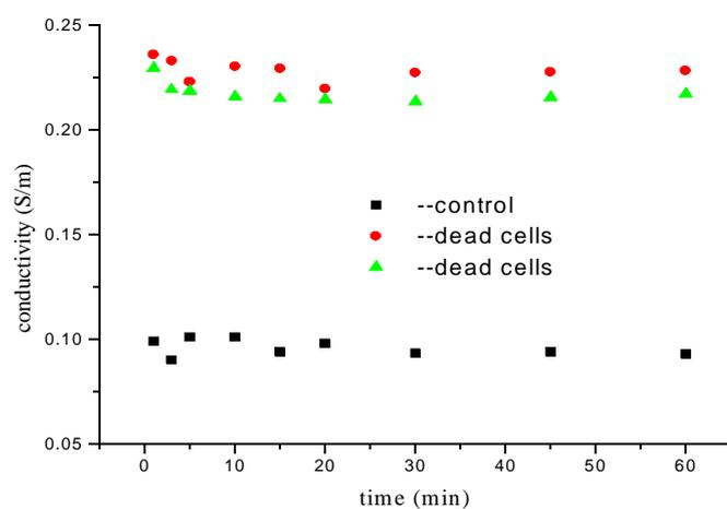
Fig. 7 Conductivity of cell suspensions containing dead cells.
