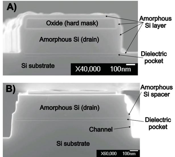
Fig. 4. SEM cross sections of the active pillar A) after the deposition of the thin amorphous Si layer (see figure 3c) and B) after channel dry etch (see figure 3d); the channel anisotropic dry etch was performed in HBr plasma with electrode power = 60W.
