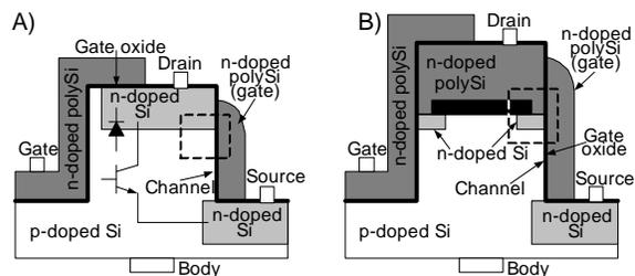
Fig. 1. Comparison of schematic cross-sections of vertical nMOSFETs with ion implanted source and drain: conventional structure (figure A) and device incorporating a DP (figure B).
