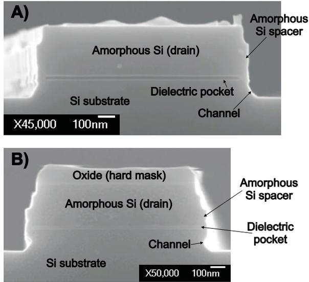
Fig. 5. SEM cross sections of the active pillar after channel anisotropic dry etch (see figure 3d) with different electrode power (P); P = 30W (figure A) and P = 100W (figure B).
