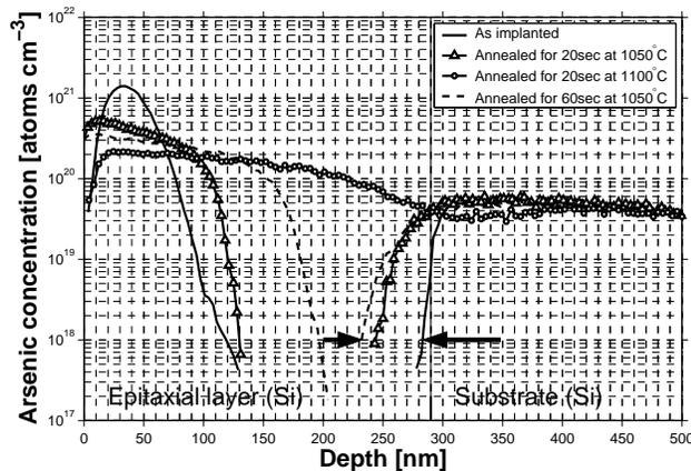
Fig. 8. SIMS profile for evaluation of As diffusion induced by RTA anneal in monocrystalline silicon grown by epitaxy without polySi cap (figure 6B); the arrows indicate As outdiffusion from the buried layer for an anneal at 1050°C for 60 seconds.
