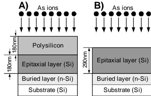
Fig. 6. Test structures fabricated in order to compare As diffusion with (figure A) and without (figure B) polySi cap layer.
