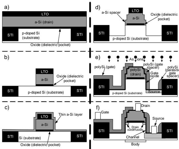
Fig. 3. Process flow of the novel fabrication process of VMOSFETs incorporating a DP.
