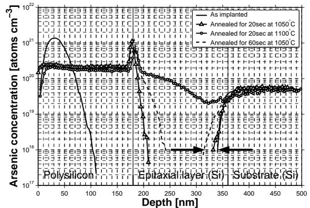
Fig. 7. SIMS profile for evaluation of As diffusion induced by RTA anneal in a test structure with polySi drain layer on top of monocrystalline silicon grown by epitaxy (figure 6A); the arrows indicate As outdiffusion from the buried layer for an anneal at 1050°C for 60 seconds.
