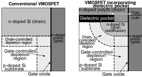
Fig. 2. Drain/channel junction of a VMOSFET incorporating DP and of a conventional VMOSFET; the figure shows the gate-controlled and the drain-controlled depletion regions in the body, assuming on-state operation ( $V_D > 0$  and  $V_G > V_t$ ); the regions represented correspond to the dotted lines in figure 1
