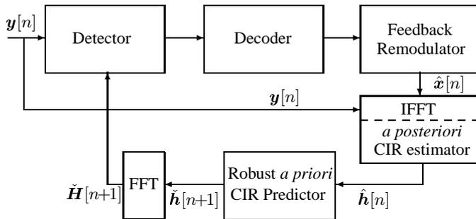
Fig. 1. Schematic of the channel estimator constituted by an *a posteriori* decision-directed CIR estimator, based on frequency-domain modulated symbol estimates, followed by an *a priori* CIR predictor.
